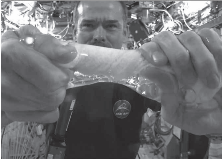
Figure 5. ISS Expedition 35 Commander Chris Hadfield explores the behavior of liquids in space by squeezing a wet cloth. Rather than dripping downward, the water wraps around Hadfield's hand like a glove made of gel (2013). Courtesy of Canadian Space Agency and NASA.
