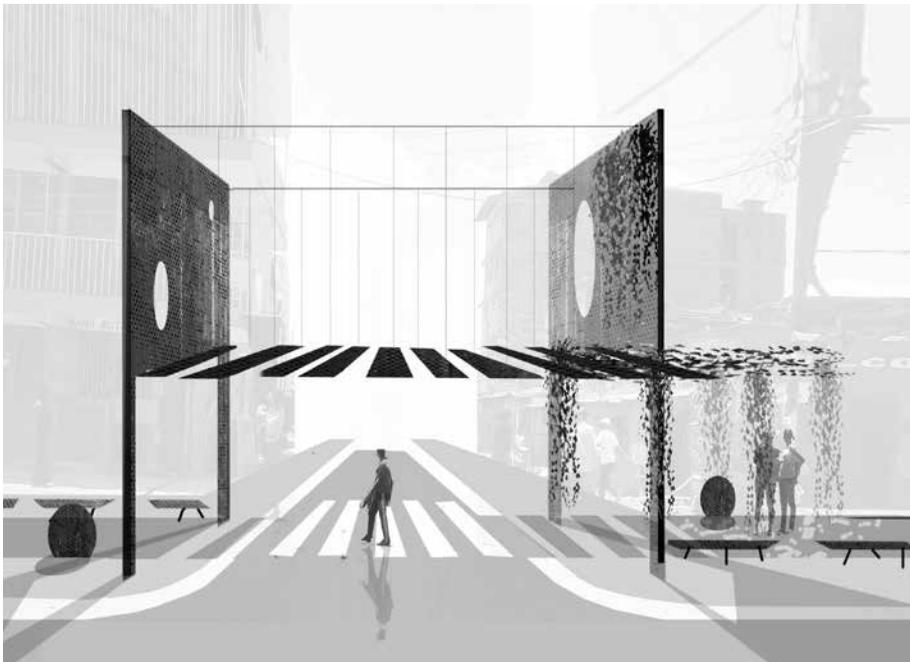
Figure 3. Initial gateway proposal. According to Cave Bureau, the design was slightly modified based on discussions regarding the branding of the project. For example, the two side squares were replaced by two triangles that represent the letter D for Dandora. Courtesy of Cave Bureau.
